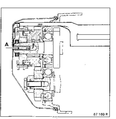
Fit a wooden block between the 5th gear fork and the drive gear for support; then remove the fork roll pin using tool **8.Vi. 31-01**
