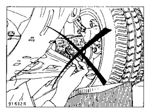
Press the brake pedal several times to bring the pistons into contact with the pads.
