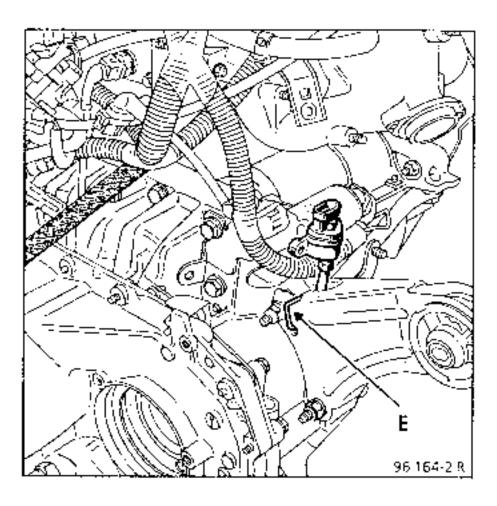
Uncouple the gear box control from the gear box output lever having removed the protective gaiter.
