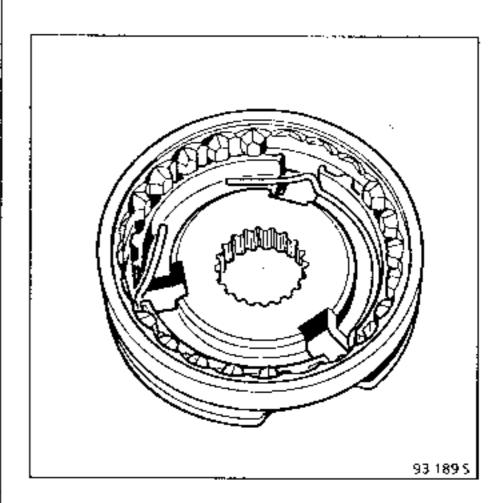
Fit the bell section of the tool on the sliding gear, turn it to the stop then extract the hub.
