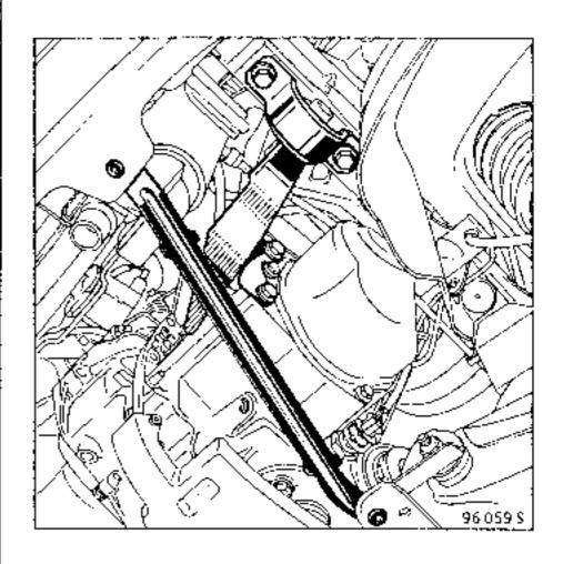
Separate the assembly from the passenger compartment and lower it so that the gear box may be uncoupled from the engine, then tilt it to remove it from the vehicle.
