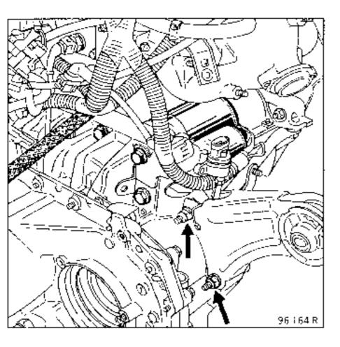
Remove studs (A) and (B) with a nut and locking nut, using an extension wrench and a ball joint socket.
