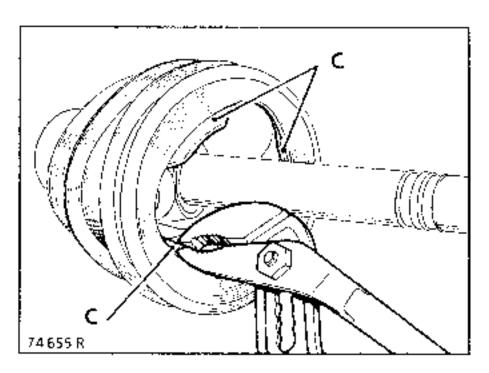
Do not remove the rollers from their bearings since each roller and needle assembly is paired and should not be inverted.
