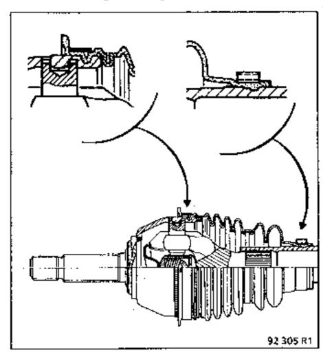
Move the joint by hand to check the two ends are correctly fitted and to ensure the correct amount of air is present in the gaiter.
