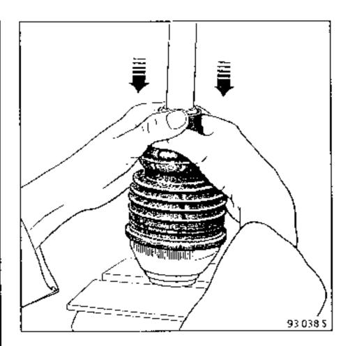
Position the edge of the gaiter correctly.
