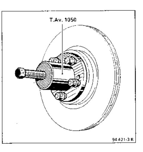
Remove the lower shock absorber base mounting bolt and extract the drive shaft.
