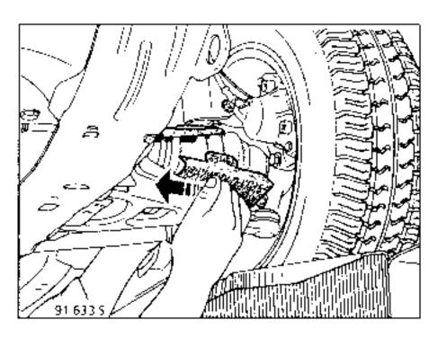
Never use a sharp tool which could damage the gaiter.
