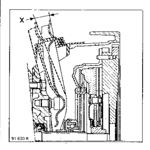
Pull the cable at the clutch fork on the gear box.
