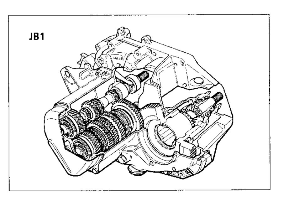
C06 vehicles are fitted with a JB type gear box.
