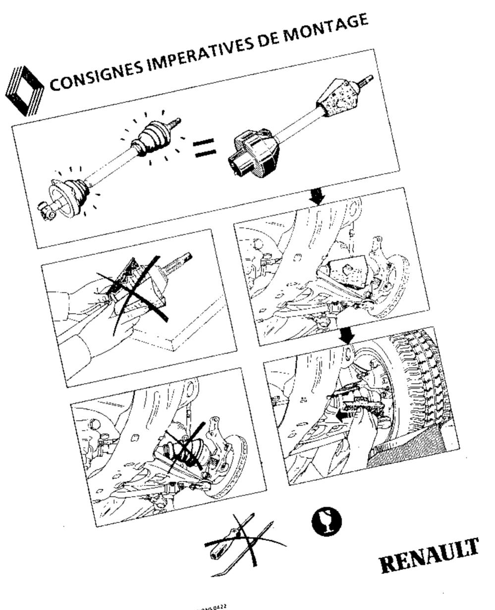
Never remove the cardboard protectors before completing the refitting of the drive shaft onto the vehicle.
