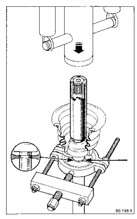
Refit the triaxe component on the splined shaft and replace the retaining circlips (depending on assembly).
