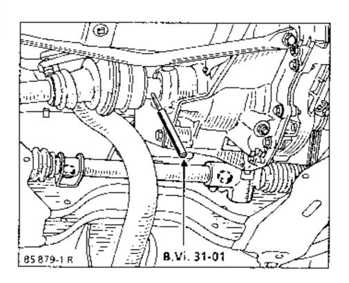
Undo the lower shock absorber base bolt (3) and remove the upper bolt
