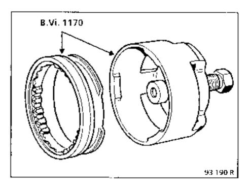
Fit the sliding gear of tool **8.Vi. 1170** as for selecting 5th gear and turn it to align the splines of the sliding gear and the hub.
