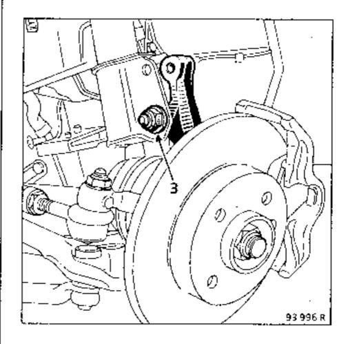
Tilt the stub axle carrier and uncouple the drive shaft
