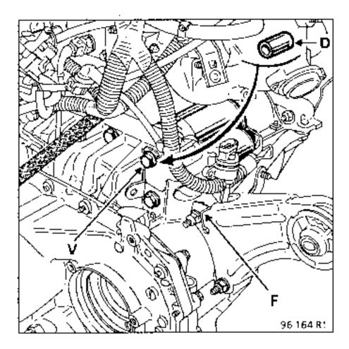
Reconnect the speedo cable ensuring pin (F) is correctly positioned.
