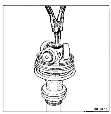
On the press, remove the triaxe component, using an extractor of type Facom US3G.
