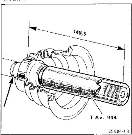
To avoid damaging the bearing which includes a lip seal, which may cause leaks, do not knock the bearing on with a hammer, but use the press to ensure progressive pressure is applied.
