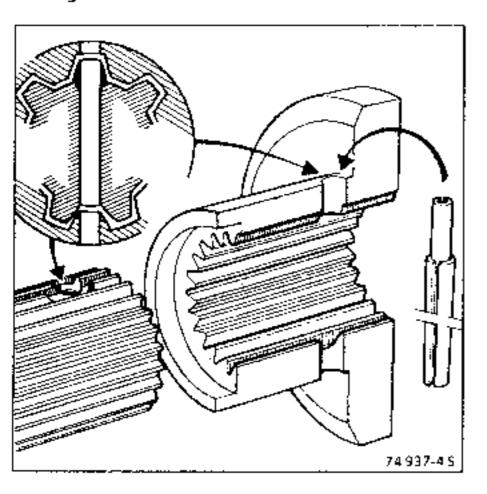
A chamfer on the sunwheel input side aids fitting the new roll pins.
