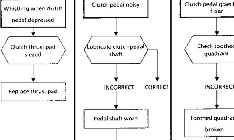
Replace the shaft and the clutch pedal bearings
