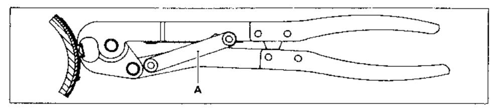
Place bar (A) in the lower notch position and close the pliers. The pre-crimped collar slides onto the gaiter and may then be positioned.
