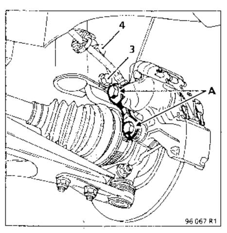
Attach the brake caliper to the suspension spring in order to avoid damaging the brake pipe.
