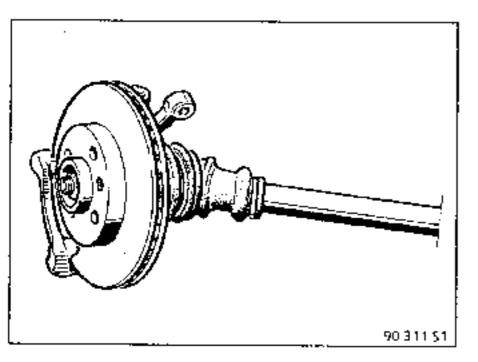
Check that the drive shaft rollers do not come out by hand. If they do, check that the needles have not fallen into the unit when refitting. From the right hand side of the vehicle, remove the drive shaft roll pins using tool 8. Vi. 31-01.
