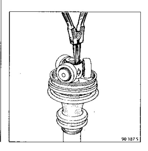
On the press, extract the triaxe component, using an unblocking and extraction tool
