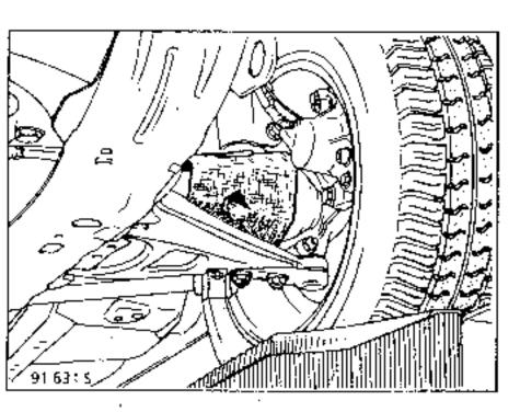
When the vehicle is on the ground, remove the cardboard protectors as shown in the diagram.
