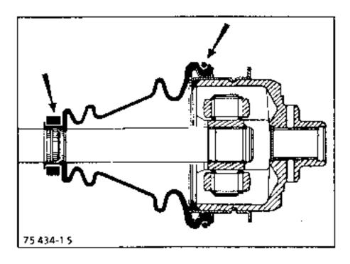
Insert a round - ended rod between the gaiter and the yoke in order to ensure the amount of air inside the gaiter is correct
