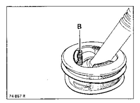
Position the lips of the gaiter in the drive shaft groove and the groove on the metal cover.
