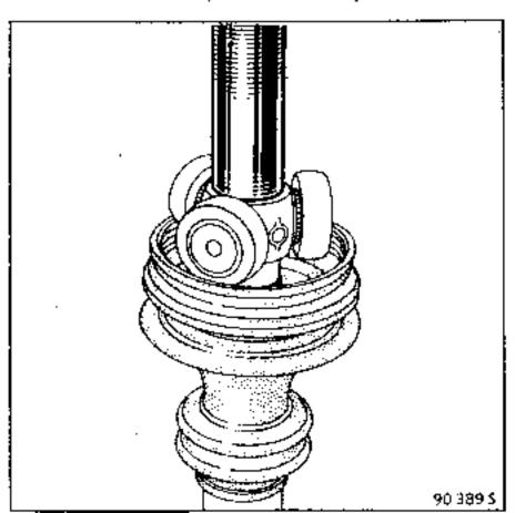
Refit the retaining circlips or crimp three points at 120° to bend over the metal of the splines on the drive shaft
