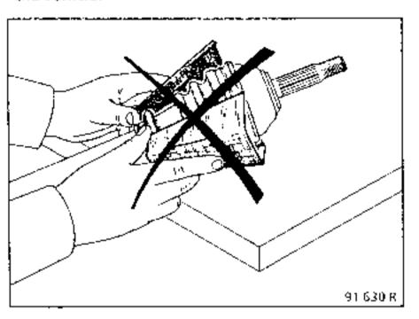
Never use a toof with a sharp edge which may damage the gaiters.
