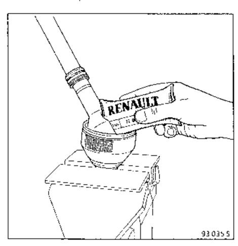
**NOTE**: the volume of grease specified in the "Consumables" section must be observed.
