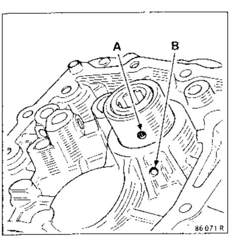
With the bellhousing resting on the tube, use the press to fit the guide tube until it comes into contact with the inner face of the bellhousing. Use tool B.Vi. 945.
