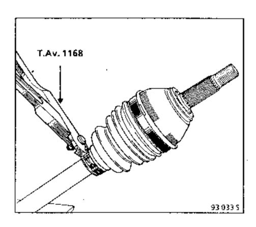
Saw off the large collar taking care not to damage the stub axle cup groove.
