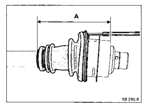
When the assembly is in this position, remove the rod.
