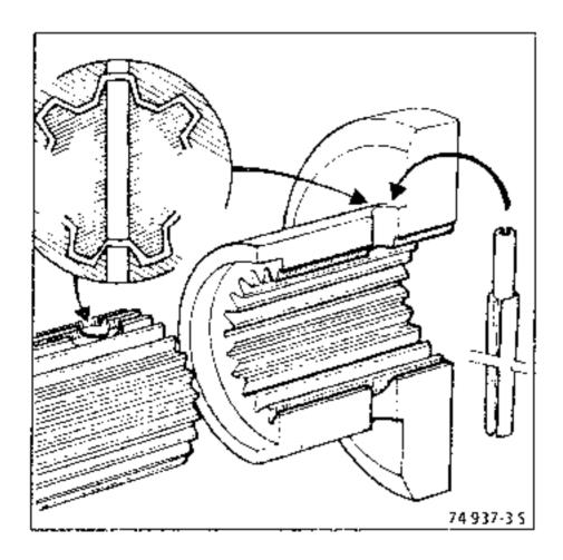
Fit new roll pins and seal the ends (CAF 4/60 THIXO).
