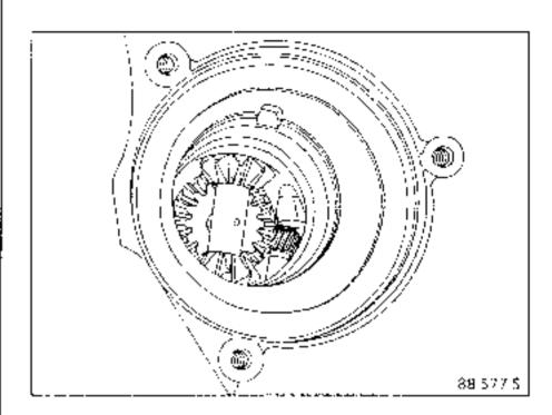
**NOTE**: The gear and the shaft should be replaced with new parts when refitting.
