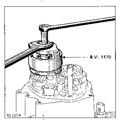
Remove the 5th gear assembly.
