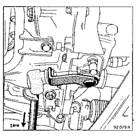
Loosen and remove the primary shaft nut and the secondary shaft bolt.
