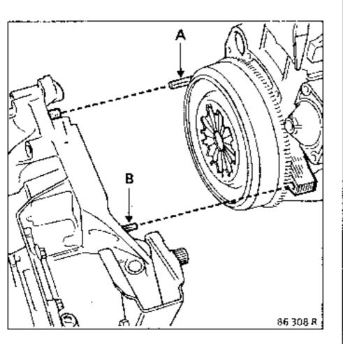
Remove the boits around the gear box and
