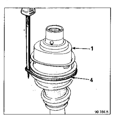
Cut the gaiter along its length and remove as much grease as possible.
