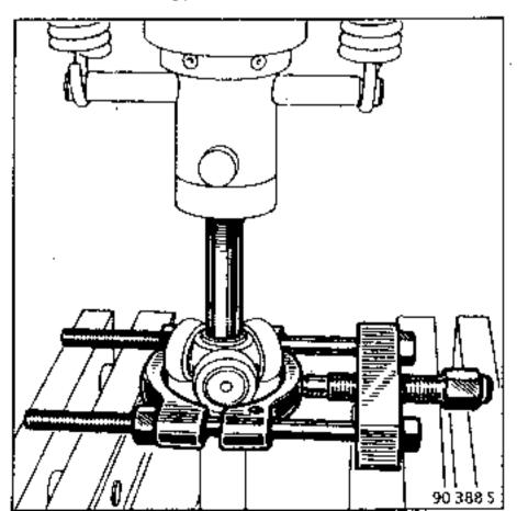
Remove the gaiter and bearing assembly in the same manner as the triaxe component.
