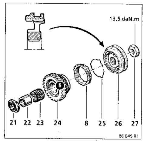
Select 1st gear with the gear lever and 5th gear in the gear box by sliding the 5th gear fork on its shaft.
