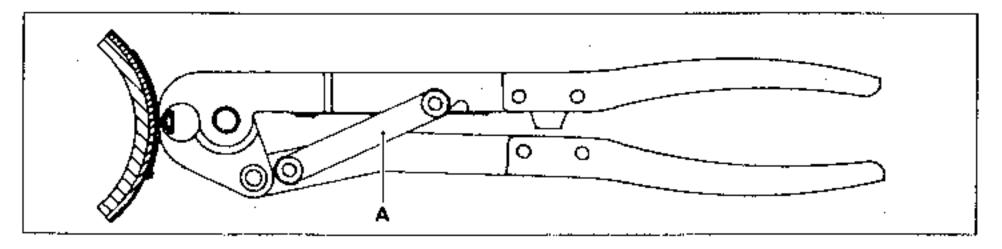
Place bar (A) in the upper notch position and close the pliers
